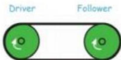
The pulleys rotate in the same direction.
