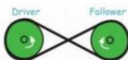
The pulleys rotate in different directions.
